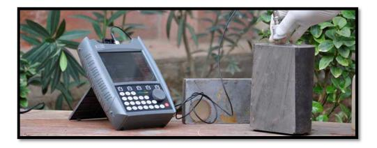
RMRC offers a variety of portable metallurgical tests for a wide range of materials. Determination of chemical analysis and material designation, hardness testing, microstructure evaluation, nondestructive testing for both metals and polymers are part of the available tests at RMRC.
